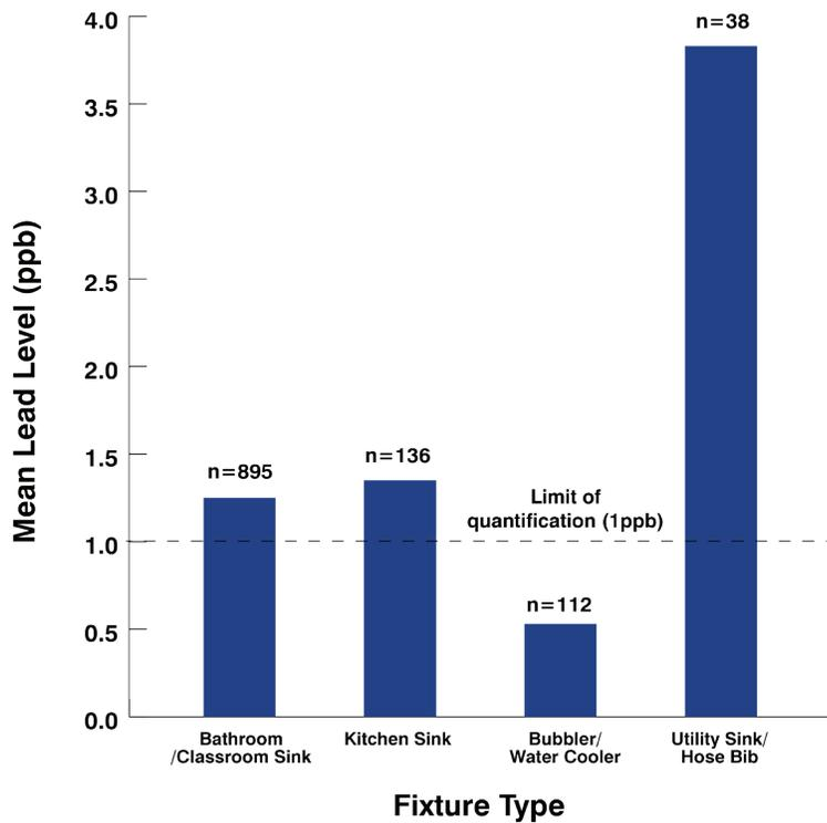
This chart illustrates the mean lead levels by fixture type for all samples (excluding those collected before LSL replacement or after fixture replacement as well as hot water samples). When levels were below the limit of quantification (1 ppb), we used 0.5 ppb.
