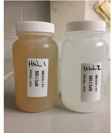
Water samples collected directly from water heater drain. Initial draw pictured on the left.
