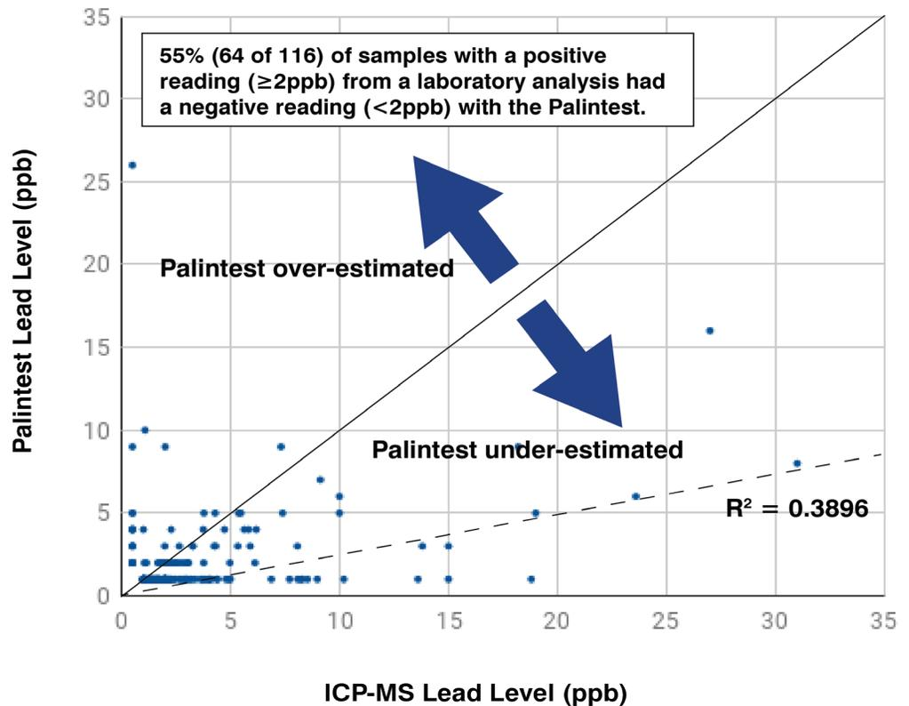
This chart compares sample results from the Palintest meter to the ICP-MS laboratory analysis. When the reading was below the limit of quantification (2 ppb for Palintest and 1 ppb for ICP-MS), we plotted the value at half the limit of quantification. The dotted line represents the observed correlation between the ICP-MS and Palintest measurements, while the solid line represents what the trendline would be if the two tests were perfectly correlated.
