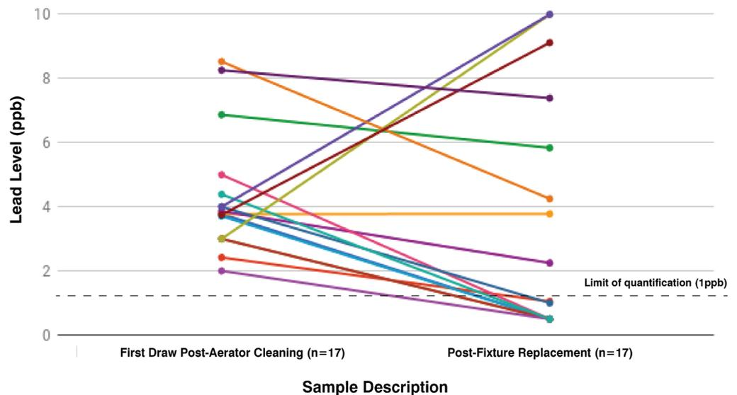
This chart illustrates lead levels at fixtures for first draw post-aerator cleaning and post-fixture replacement when the initial sample was 10 ppb or lower. Lines connect data for a single fixture. The limit of quantification for ICP-MS (1 ppb) is indicated with a dashed line; samples below the limit of quantification are plotted at 0.5 ppb.
