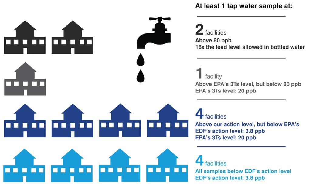
Results of water testing (excluding samples from utility sinks and hose bibs) at 11 child care facilities: two facilities had at least one tap water sample above 80 ppb level of lead; one facility had at least one sample above EPA's 3Ts action level of 20 ppb, but below 80 ppb; four facilities had at least one sample above our health-based action level of 3.8 ppb, but below 20 ppb; and 4 facilities had all samples below EDF's action level of 3.8 ppb.
