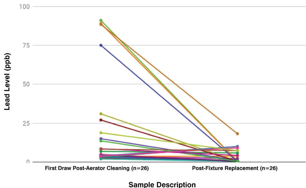
This chart illustrates lead levels at fixtures for first draw post-aerator cleaning and post-fixture replacement. Lines connect data for a single fixture.
